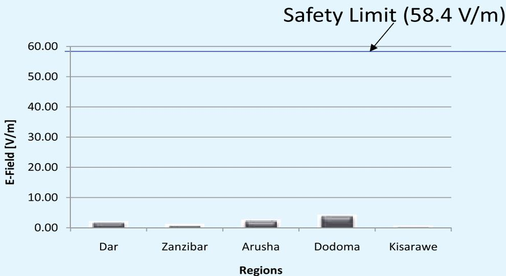
Fig. 9. Maximum E-field measured in different regions at GSM 1800 frequency band. The solid blue line indicates the safety limit of exposure for this frequency
